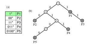
Figure 1: a) routing table, b) corresponding binary trie.
